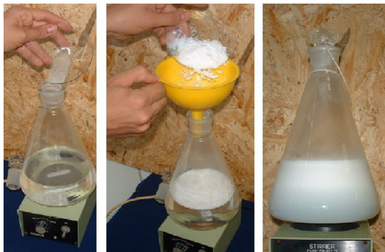
Figure 3.13: Main stages of FOCUS suspension preparation: dosage of SDS, dosage of powder, stirring, and the ready-to use suspension (thick creamy layer can be seen forming on the top) [133].
