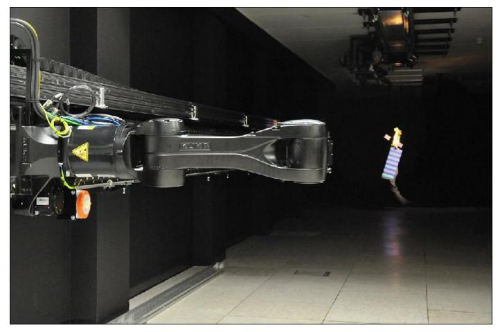
GRALS Testbed. This robotic arm, attached to a 33 m track is ESA's GRALS (GNC Rendezvous, Approach and Landing Simulator), is part of the Agency's Orbital Robotics and Guidance, Navigation and Control Laboratory. GRALS is used to simulate close approach and capture of uncooperative orbital targets, such as drifting satellites or to rendezvous with asteroids. It can also be used to test ideas for descending to surfaces, such as a lunar or martian landing (image credit: ESA, M. Grulich)
