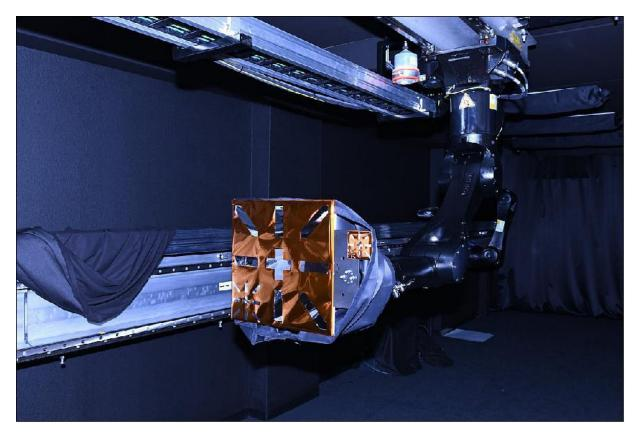
Initial testing of these 'Passive Emitting Material at end-of-life' or PEMSUN markers took place at the end of March 2019 inside ESA's <u>GNC Rendezvous</u>, <u>Approach and Landing Simulator</u>, part of the Agency's Orbital Robotics and Guidance, Navigation and Control Laboratory, at its ESTEC technical center in Noordwijk, the Netherlands (image credit: ESA)
