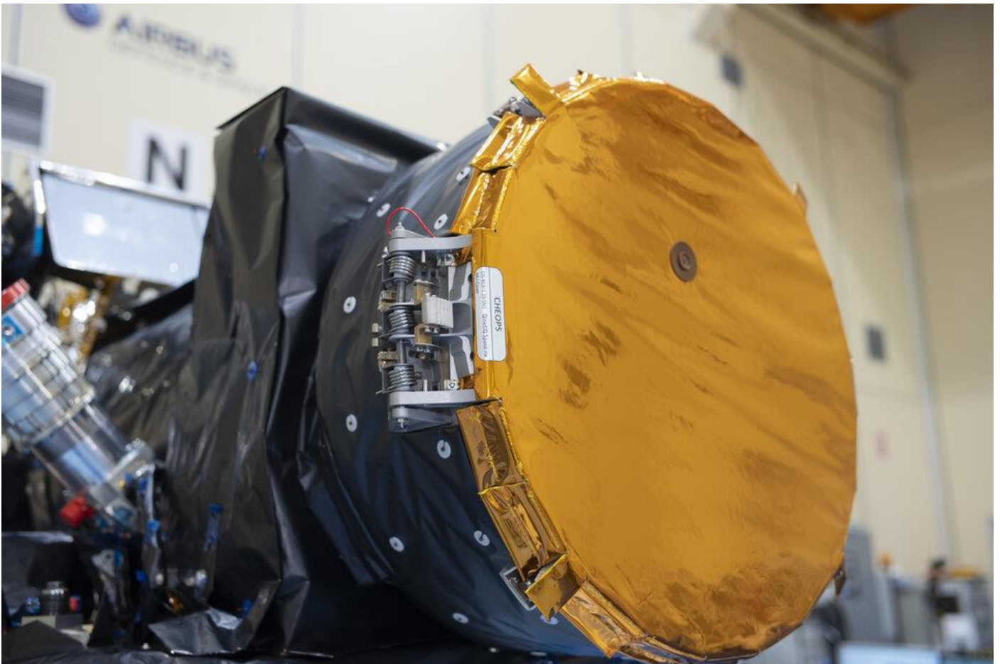
The baffle cover of Cheops in the clean room
