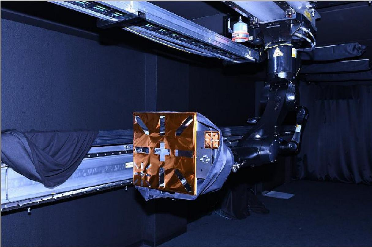
**Initial testing of these 'Passive Emitting Material at end-of-life' or PEMSUN markers took place at the end of March 2019 inside ESA's [GNC Rendezvous, Approach and Landing Simulator](#), part of the Agency's Orbital Robotics and Guidance, Navigation and Control Laboratory, at its ESTEC technical center in Noordwijk, the Netherlands (image credit: ESA)**
